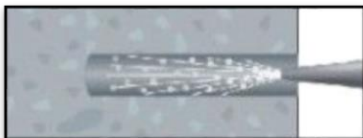
Step 2: Clean the drill hole
