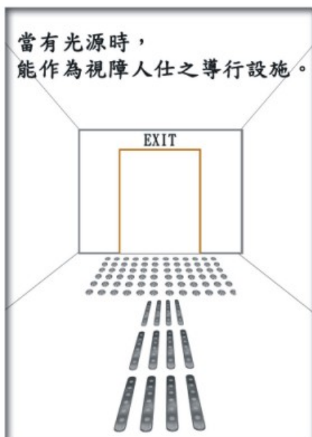
In normal situation, Sunway Glow Cap Tactile System can be the tactile guide for visually impairer.
