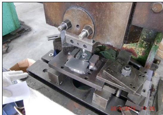
Stamping machine for production of steel tubes
