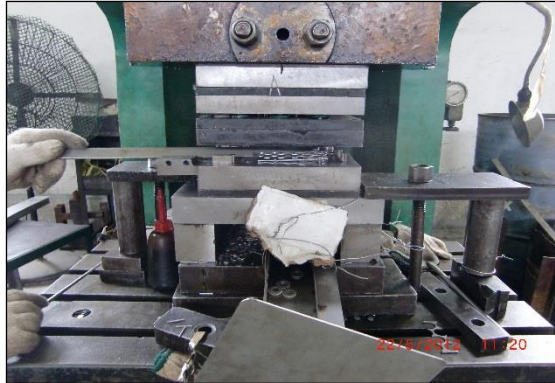
Stamping machine for production of washers
