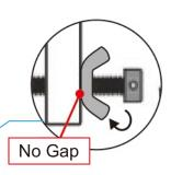
Tighten up the screw. By using visual inspection, ensure there is no gap between the stone lifter and stone surface. And then, tighten the safety wing nut. Afterwards, slightly lift up the stone to conduct the double-check.
