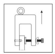
After ensure the stone has been fixed by stone lifter, can fully lift up the stone panel.
